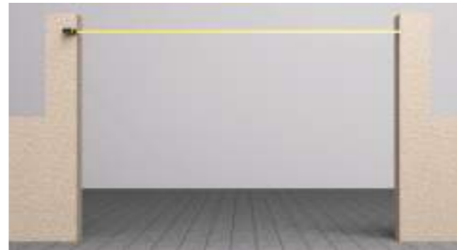
5 Mesurer en haut. Retenir la plus petite mesure; Measure at the top. Retain the small plus measure;
